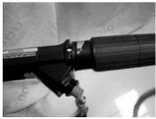
5. Pull out the choke knob fully.
