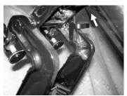
3. Loose the steering friction adjuster by turning it counterclockwise, and adjust the steering friction according to operator preference.
